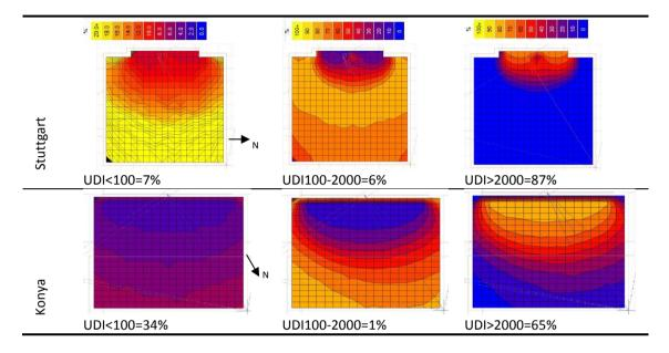
Figure 5: Useful Daylight Illuminance comparison.
