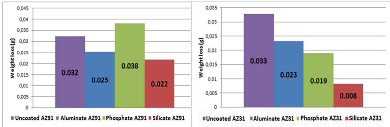
Fig. 4. Weight losses (g) of the AZ31 and AZ91 samples after 96 hours.
