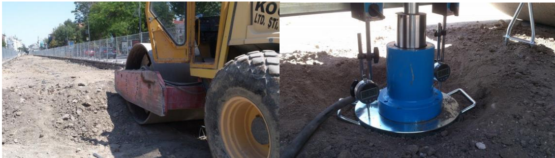
Figure 6. Plate Loading Experiment
