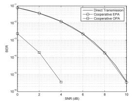
Fig. 5. BER for relay-assisted VLC schemes with EPA and OPA. No lighting constraint is considered.
