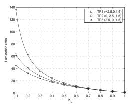
Fig. 3. Luminance ratio between the task and the test points versus  $K_L$ .
