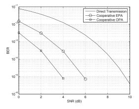
Fig. 6. BER for relay-assisted VLC schemes with EPA and OPA with lighting constraints
