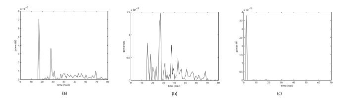
Fig. 4. The channel impulse responses for the (a)  $S \rightarrow R$  link  $c_{sr}(t)$  (b)  $S \rightarrow D$  link  $c_{sd}(t)$  (c)  $R \rightarrow D$  link  $c_{rd}(t)$ .
