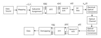
Fig. 1. O-OFDM transmission block diagram.
