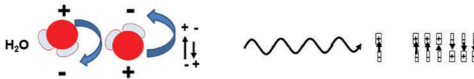
Figure 4. Due to bipolar structure of water molecules, ions in the cells and in inter-cellular space are heated up.
