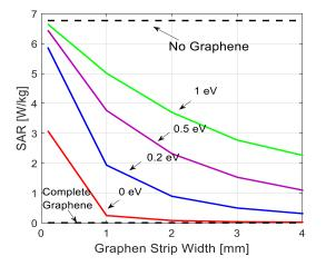
Fig. 9. SAR at 30 mm from the feedline vs. the width w of the graphene strip, for different level of chemical potential.
