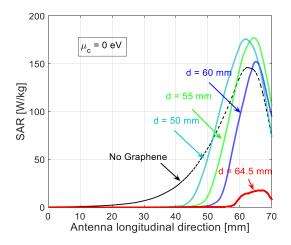
Fig. 8. Specific Absorption Rate (SAR) along the antenna at 1.5 mm from the outer conductor for the  $2^{nd}$  configuration for different distances between graphene and the slot. The feedline is at 0 mm and the slot is located at 65 mm.
