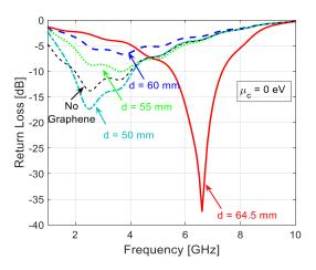
Fig. 7. Return loss obtained with the second configuration for different distances between the graphene and the slot.
