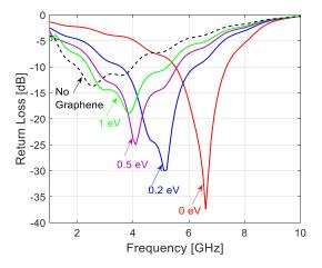
Fig. 5. Return loss obtained with and without graphene sheet for different chemical potential level.
