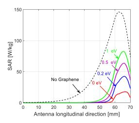
Fig. 6. Specific Absorption Rate (SAR) along the antenna at 1.5 mm from the outer conductor for the 1<sup>st</sup> configuration where the graphene cover all the way from
