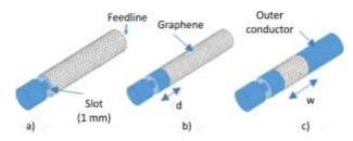
Fig. 4. Microwave coaxial antenna with the graphene sheet: (a) antenna fully covered by the graphene sheet from the slot all the way to the feedline; (b) graphene shifted from the slot and covering all the way to the feedline; (c) graphene strip shifted from the slot.
