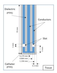
Fig. 3. Schematic 2D view of the microwave coaxial antenna in the biological tissue (not drawn to scale).
