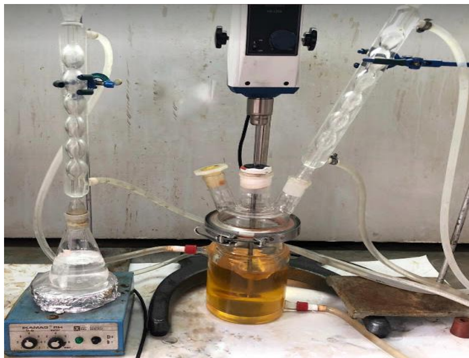
Figure 1. Pre-activation of the catalyst and transesterification of waste cooking oil
