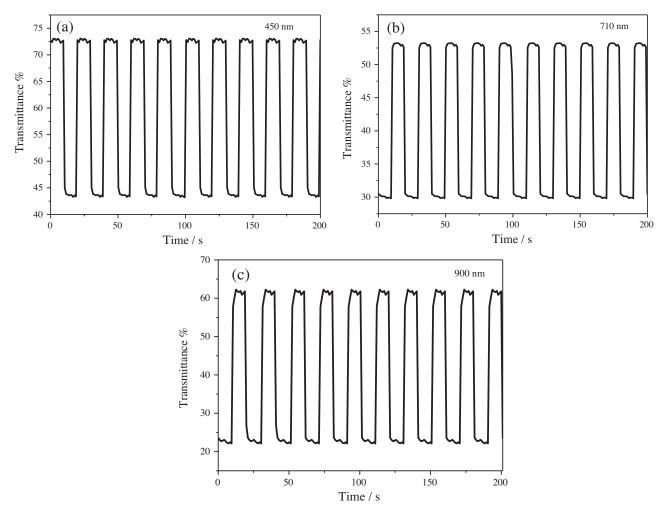
**Figure 5**. Chronoabsorptometry experiments for P(DTP-alkoxy-DTP) (25 cycled) at (a) 450 nm (b) 710 nm, and (c) 900 nm in 0.1 M TBAPF<sub>6</sub>/ACN during the switching of the polymer film in 10 s between 0.0 V and 1.1 V vs Ag wire.
