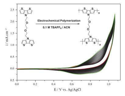
$\textbf{Figure 1}. \ \ \text{Electrochemical polymerization of DTP monomer in 0.1 M TBAPF}_{\,6}/\text{ACN solution on an ITO electrode}.$
