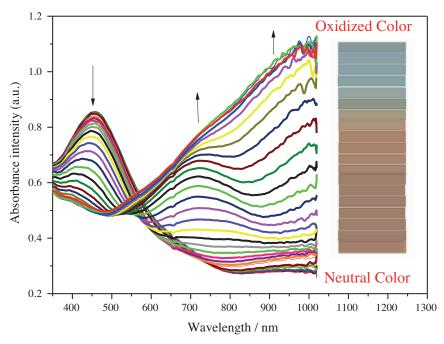
Figure 4. Electronic absorption spectra of P(DTP-alkoxy-DTP) on ITO in 0.1 M TBAPF  $_6$  /ACN.
