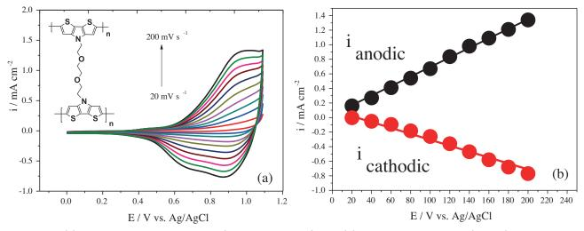
Figure 2. (a) p-Type doping behavior of P(DTP-alkoxy-DTP) film (b) relationship of anodic ( $i_{anodic}$ ) and cathodic current ( $i_{cathodic}$ ) peaks relationship of anodic ( $i_{anodic}$ ) and cathodic current ( $i_{cathodic}$ ) peaks at various scan rates in 0.1 M TBAPF <sub>6</sub>/ACN.
