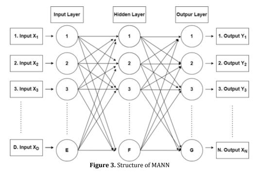
In Figure 2, each cell in the hidden and output layers takes the NET-weighted total outputs from the previous layer as input. NET values are found in Eq. 2.
